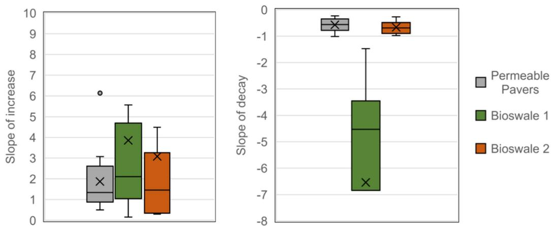
Fig. 11. Slope coefficients of the increase and decay of the effluent temperatures.
