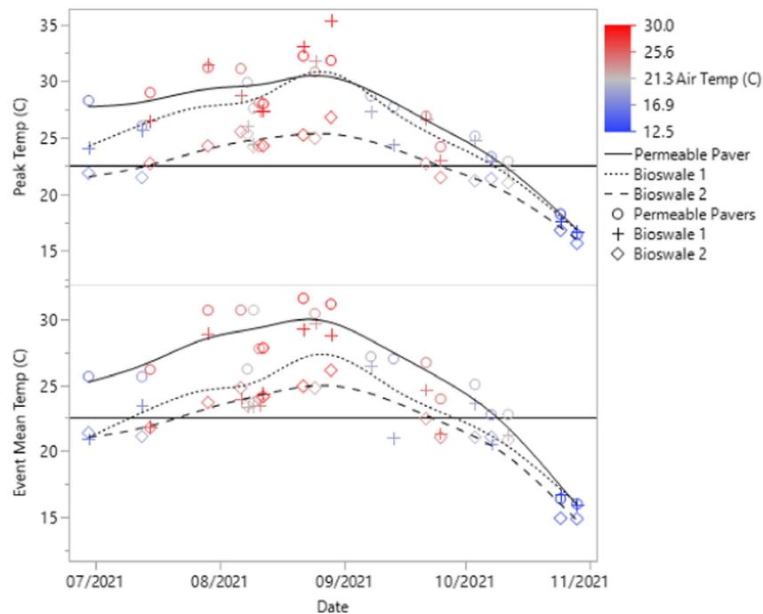
**Fig. 8.** Peak temperature and event mean temperature as a function of the date. The ambient air temperature for each event is represented by the color bar and the horizontal line represents the minimum mean temperature threshold for freshwater species (22.5°C).
