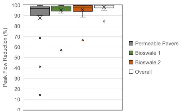
**Fig. 5.** Distribution of the peak flow reduction in each green infrastructure practice and the overall system.
