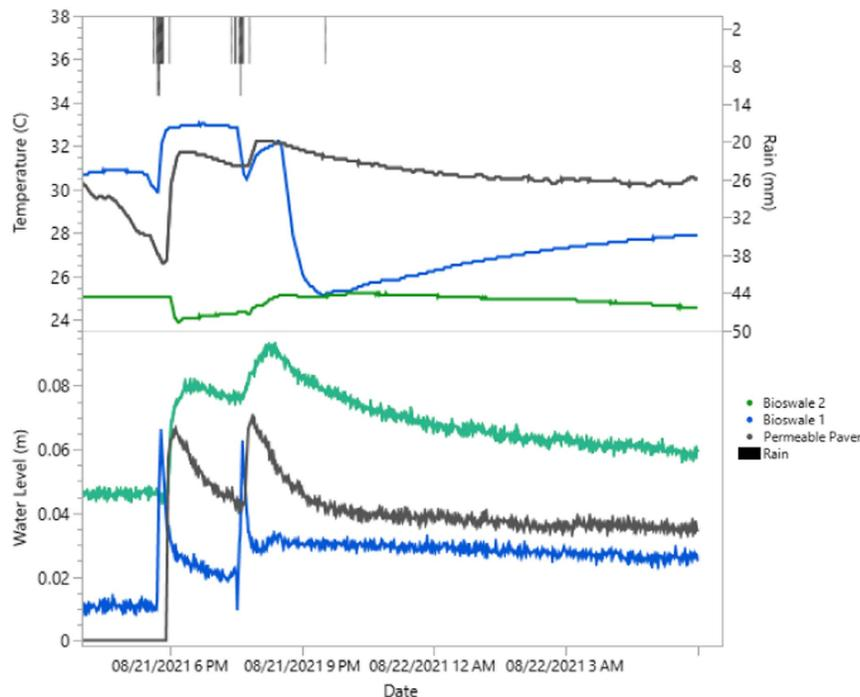
**Fig. 10.** Example of temperature fluctuations over the course of a runoff event.
