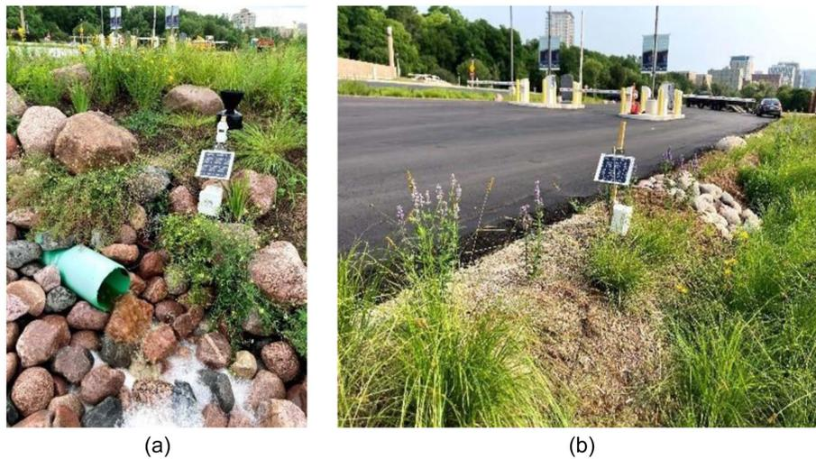
**Fig. 2.** Bioswale 2 outfall into rip-rap channel, rain gauge, and data logger (a); and data logger in Bioswale 2 that measures the discharge from the permeable paver and Bioswale 1 underdrains (b). (Images by Matthew Dupasquier.)
