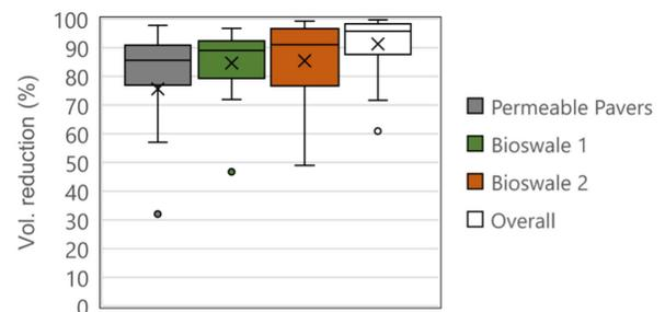
**Fig. 3.** Distribution of the percent of stormwater runoff volume per rain event that is reduced by the three green infrastructure practices and the overall system.
