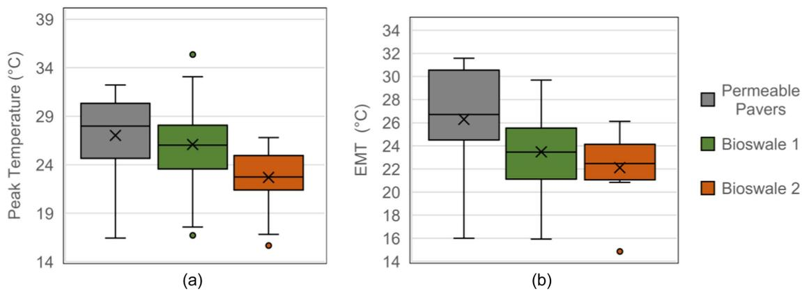
**Fig. 7.** Distribution of the peak temperature (a) and the event mean temperature; and (b) for stormwater runoff events captured at the underdrain of each green infrastructure practice.
