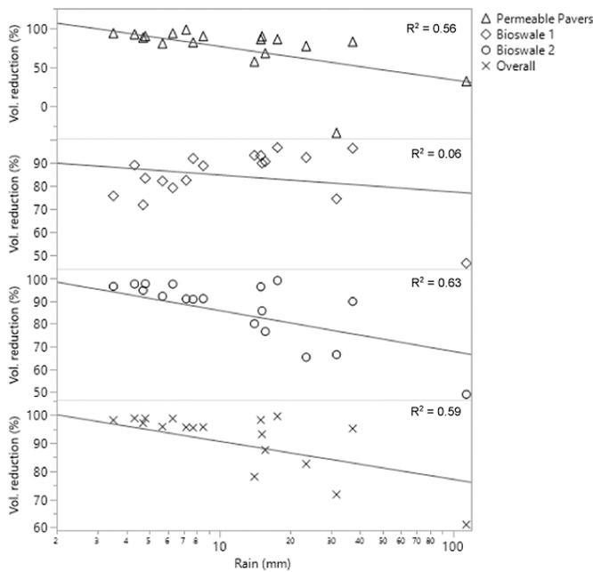
**Fig. 4.** Percent of stormwater runoff that is infiltrated as a function of rainfall depth.
