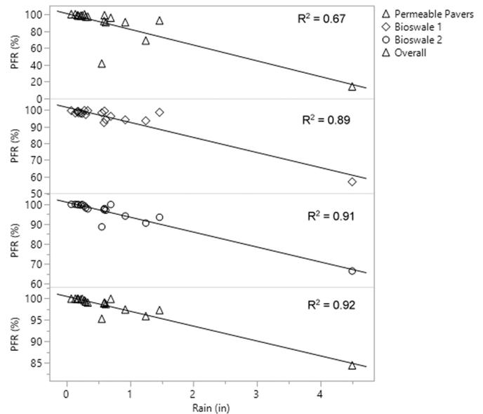
**Fig. 6.** Peak flow reduction (PFR) as a function of the rainfall depth.
