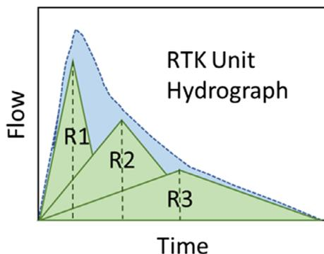
FIGURE 2. Example of an RTK unit hydrograph. The dashed blue line represents the total flow from the rainfall-derived inflow and infiltration (RDII), R1 represents the component of RDII that is attributed to quick inflows, R3 is the portion of flow that is attributed to slower infiltration, and R2 is a combination of the two.
