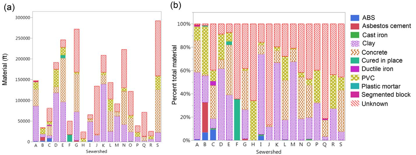
FIGURE 4. Pipe materials in each sewershed as a total length (a); and as a percentage of the overall sewershed pipe length (b).
