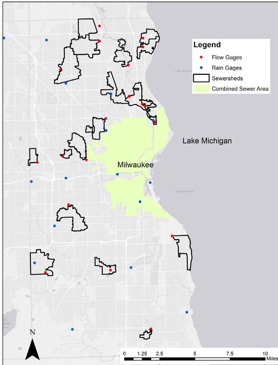
FIGURE 1. Map of the selected sewershed locations within the separated sewer system in the Milwaukee metropolitan area, as well as the location of the rain and flow gages used in the study.
