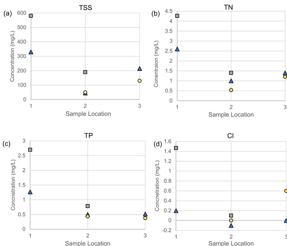
Fig. 8. The concentration at different sampling locations in the wetland for TSS (a), TN (b), TP (c), and Cl (d). With the sample locations being inlet (1), observation well (2), and outlet (3). The various shapes indicate different stormflow sampling dates.
