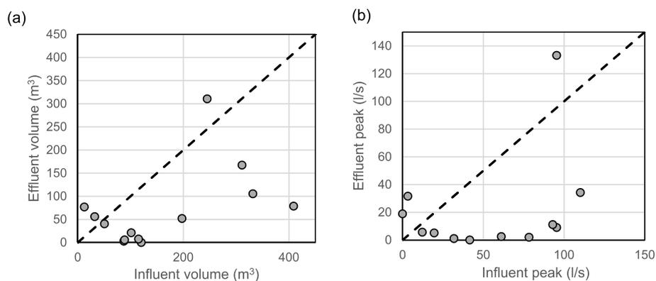
Fig. 2. Comparison of the influent and effluent volume (a) and peak flows (b), with the dashed line represented as a 1:1 relationship.
