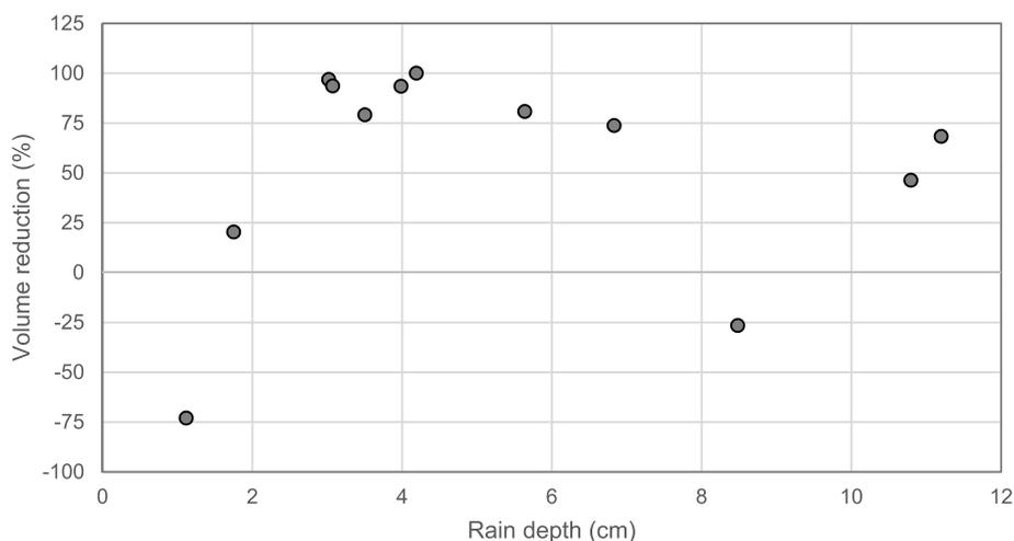
Fig. 3. The percent volume reduction over different rainfall depths. Not illustrated is the low outlier at 0.4 cm that had a negative volume removal.
