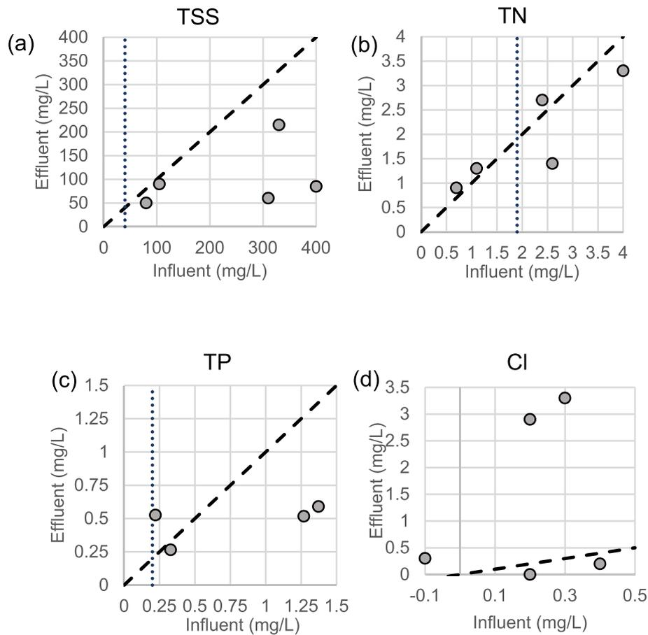
Fig. 5. Influent and effluent concentrations in the wetland for (a) TSS, (b) TN, (c) TP, and (d) Cl. With TSS, TN, and TP also containing vertical lines which represent the irreducible concentration.
