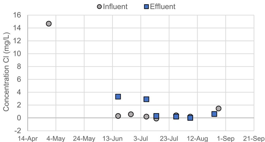
Fig. 7. The influent and effluent concentration of Chloride in the wetland over time.
