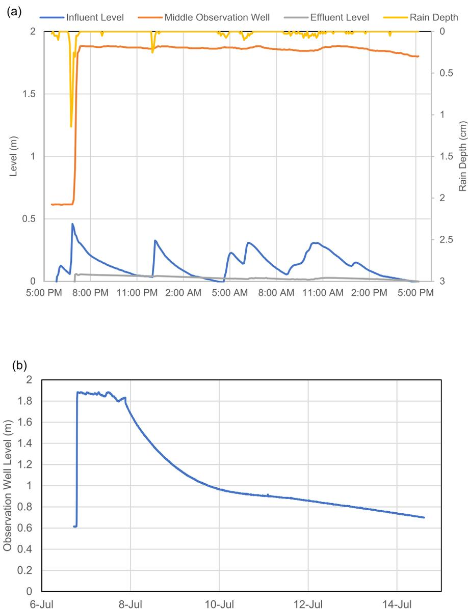
**Fig. 4.** The level of influent, effluent, and middle observation well and the rain volume (a), and the level of the middle observation well (b), are shown over time for a single storm event.
